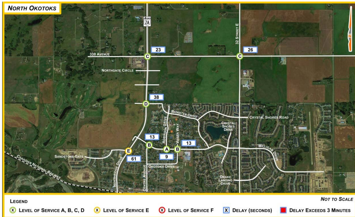
Figure 3.15 a 2035 Improved Intersections Operational Conditions – North Okotoks
