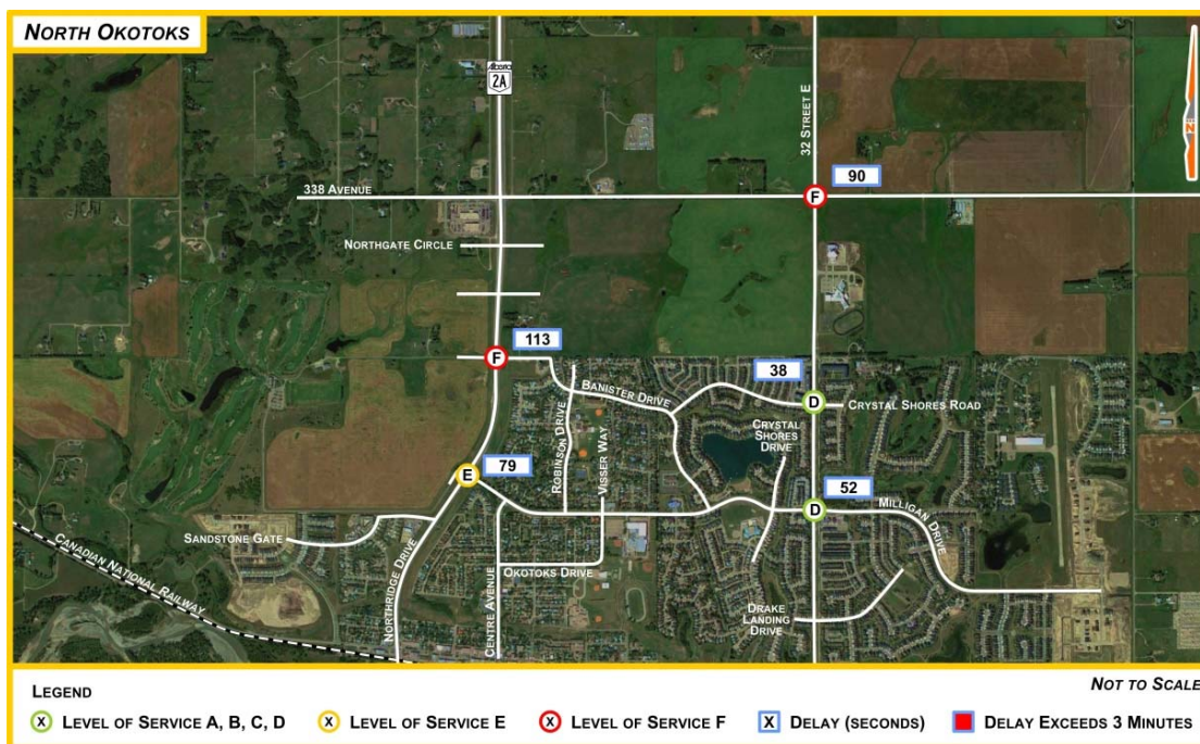
Figure 3.19 a 2045 Improved Intersections Operational Conditions – North Okotoks
