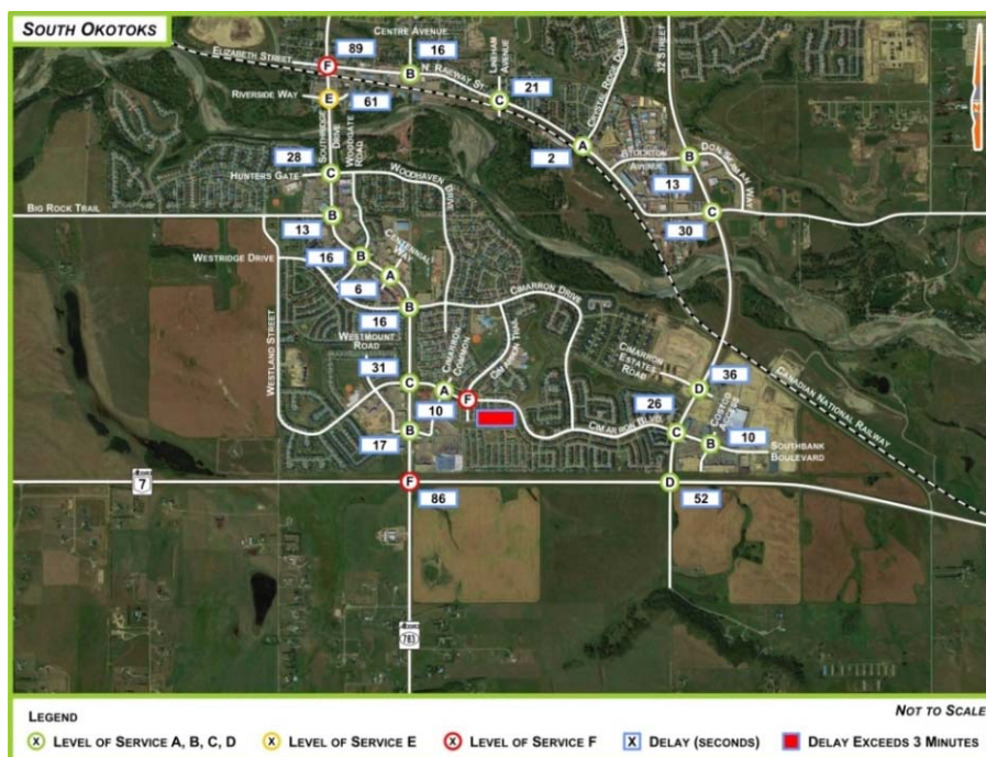
Figure E 3.10 b 2035 Operational Conditions – South Okotoks
