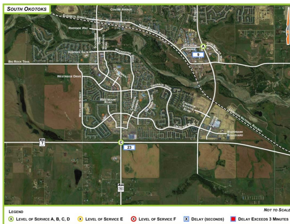
Figure 3.11 b 2025 Improved Intersections Operational Conditions – South Okotoks
