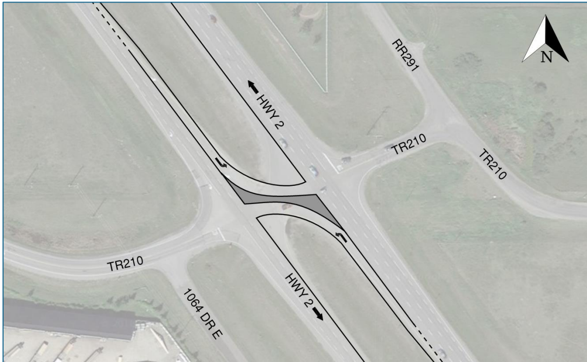
Figure 13: Turn Restrictions Using Directional Median Opening
